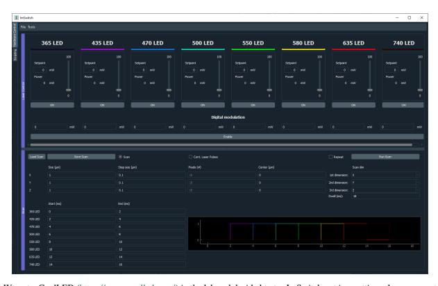
We got a CoolLED (https://www.coolled.com/) in the lab and decided to try ImSwitch out in a setting where we want to control the 8 lasers of the device, both by doing it manually using the sliders and buttons (using a USB port and RS232 communication protocol), but also being able to design and perform a sequence of TTLs and a X-Y-Z Stage controlled by a National Instruments card. This use case could be combined with the Napari viewer and a camera, or
